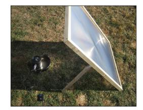
In this picture, you can see that I'm using a remote cooking thermometer. On an 18 degree day, it took 10 minutes and 28 seconds to heat the water from 58 degrees to 158 degrees. The lid being cracked made a BIG difference. The next time I did it, I didn't use a thermometer and the lid stayed closed. As a result, the temperature of the water was 177 degrees after 9 minutes. A few more minutes, and I would have had boiling water and I could have drawn off the steam a had distilled water.
